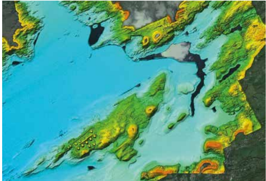
Fig. 6.6 Seamless integration of offshore multibeam data and terrestrial/intertidal LiDAR bathymetry data in Bantry Bay, Ireland, superimposed in Google Earth.
